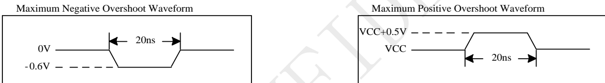
Figure 5-1 Maximum Overshoot Waveform
